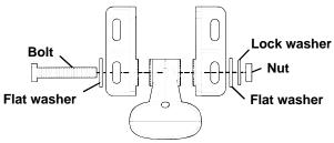
Assemble transducer and bracket.
